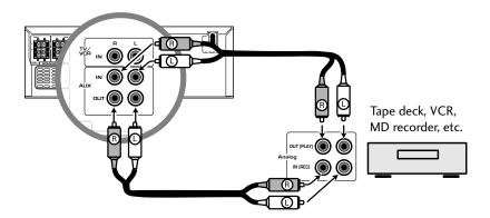
1 Use a stereo audio cable to connect the AUX IN jacks to the analog outputs of an external component.
